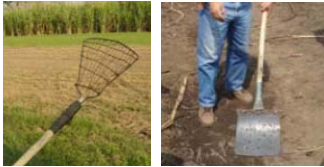
Figure 26. Devices for mechanical control when cane burning; metal structure designed by Pantaleon Sugarmill (left) and other, rubber-based, designed by La Union Sugarmill (right)
